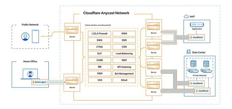
Once tunnels have been established, there are two methods for how user traffic is forwarded to your application or service. Each method below is protected by policies managed by the ZTNA service that enforces authentication and access (which will be explored in further depth later in this document).
