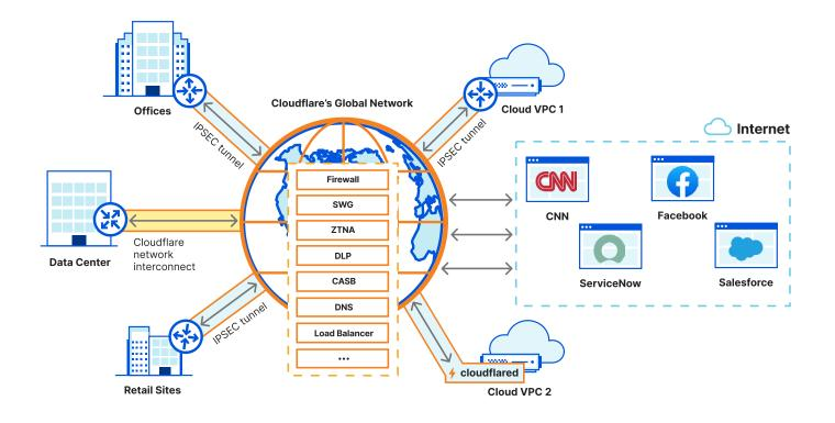
As previously described, Cloudflare uses a routing technique called <u>Anycast</u> to globally advertise all of the services and endpoints on the Cloudflare network, including the endpoints for WAN IP tunnels.
